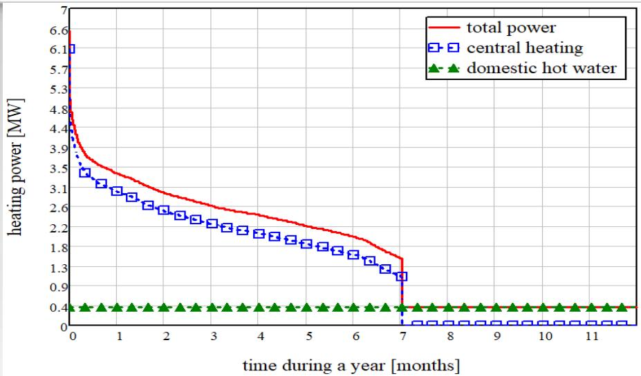
**Control of thermal power delivery - dynamic curve (heat user in the option dhGeoA)**
