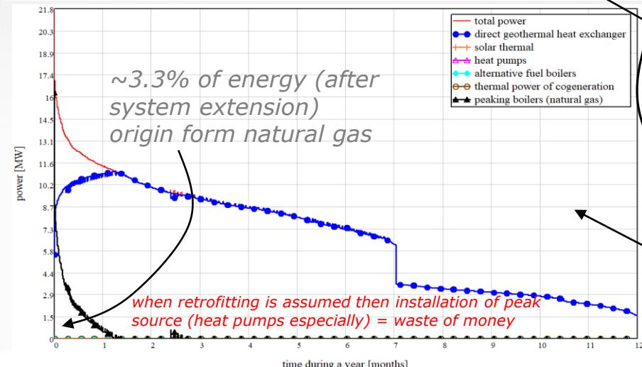
**E-xtended energy user, actual heating system (90/70/20/-20°C ), no heat pumps**
